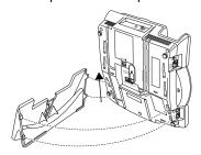
3. Align the bracket's keyhole slots with the wall plate studs, then slide the base downward to secure it.
